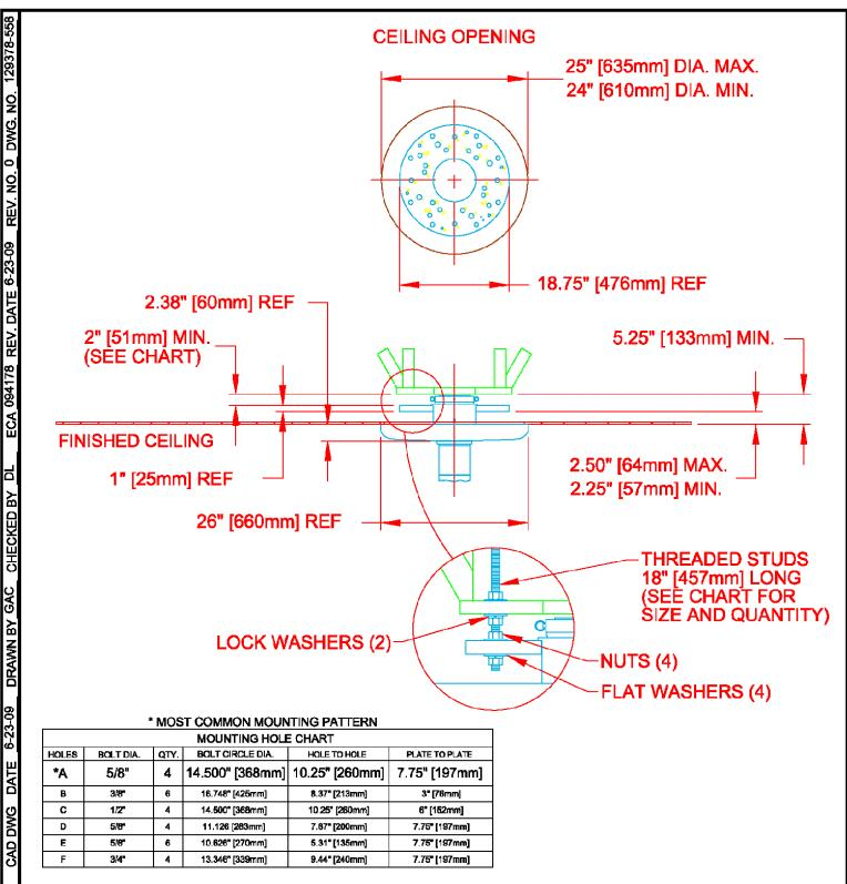
1. ALLOW EXTENSION BOLTS OR FULLY THREADED STUDS TO EXTEND 1.25"±.125" (32MM±3.2mm) THROUGH BOTTOM OF STERIS CEILING PLATE. EXTENSION BOLTS OR FULLY THREADED STUDS TO BE CLASS 2B THREAD SAE J429/ASTM A449 GRADE 5 OR ASTM A193 GRADE B7 MATERIAL OR BETTER. CORRESPONDING GRADE NUTS TO BE USED. DO NOT USE TOGGLE BOLTS. PLATE TO PLATE DIMENSION IN CHART IS MAX. FOR SEISMIC INSTALLATIONS.
