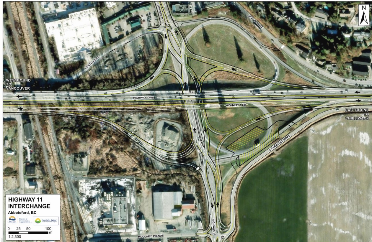
FIGURE 2: HIGHWAY 11 INTERCHANGE REFERENCE CONCEPT DESIGN
