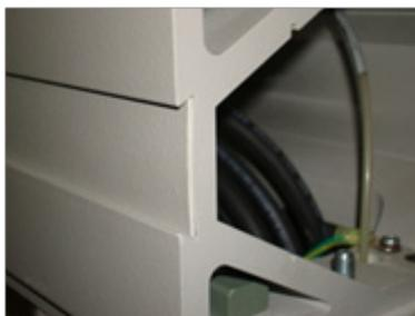
4. Slide strip in channel on boom and make sure strip is flush in channel.
