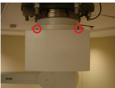
1. Remove the end cap by unscrewing the two (2) screws attaching the top portion of the end cap.
