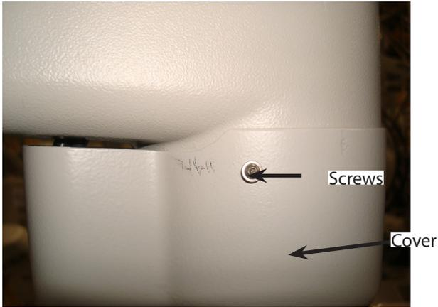
1. Remove the three screws and cover.
