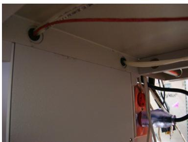
9. Remove shelf and pull air lines out of the back of the shelf.
