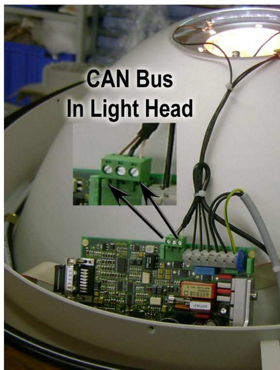
*CAN BUS Connection in the Light Head
