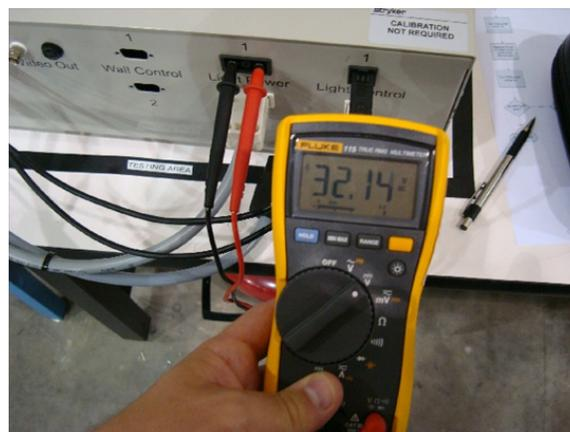
*Power Supply Box DC Voltage Measurement*
