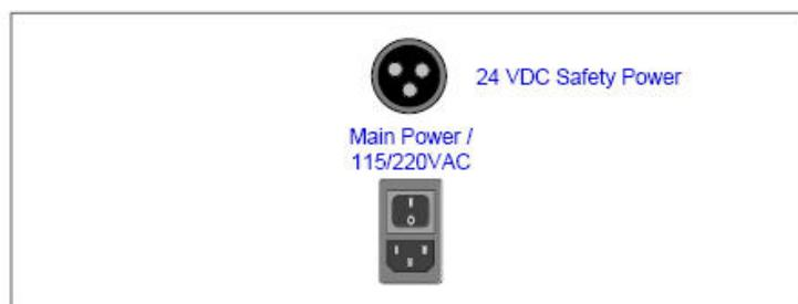
*Power Supply Box (Front and Rear View)*
