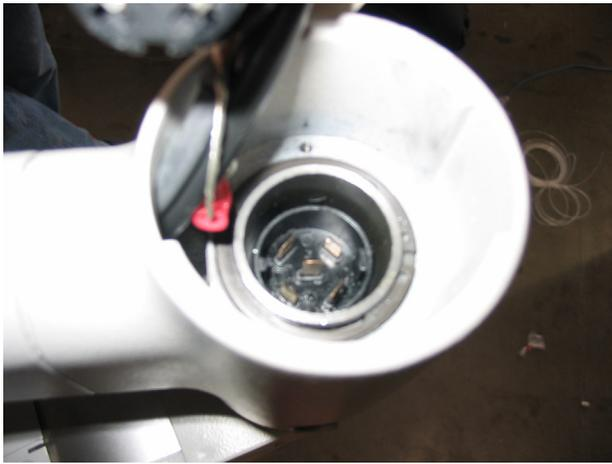
5. Insert washers into top of Suspension Arm.
