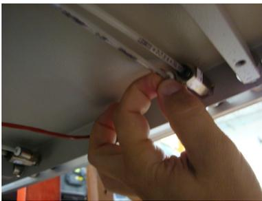
4. Label the brake lines to prevent improper reconnection.
