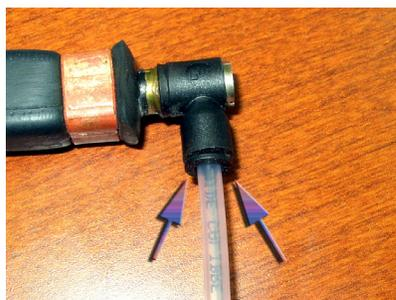
*Air release valve showing connections Brake bladder with hose connected*
