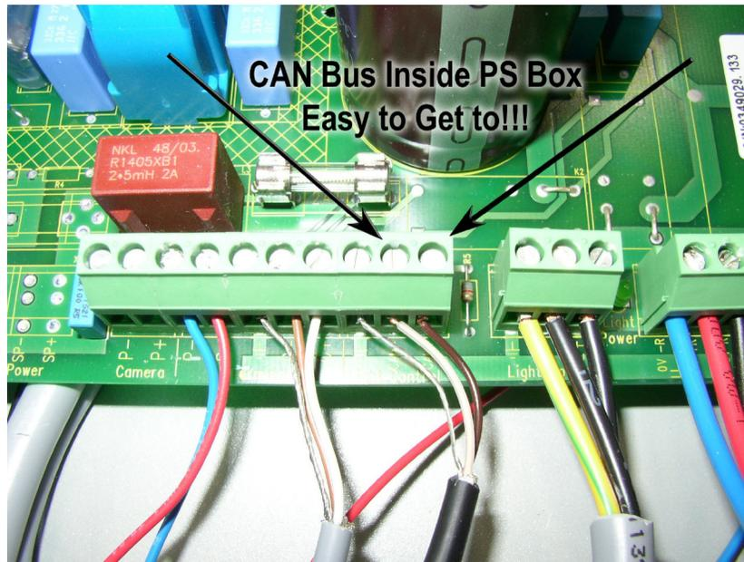
*CAN Bus connection in the power supply box on the internal circuit board
