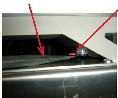
1. Insert the EP module into the arm set opening. Pay close attention to the slots allocated in the arm set to fit the EP Module box.
