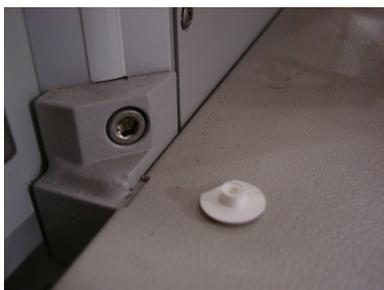
8. Remove protective caps and four screws that attached shelf to service head.
