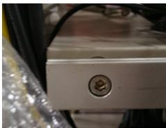
4. Loosen the four hex screws on the shelf rail.
