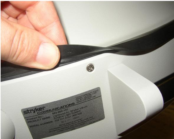
1. Remove the cover from the light head by removing the 10 Phillips head screws around the circumference of the light head.
