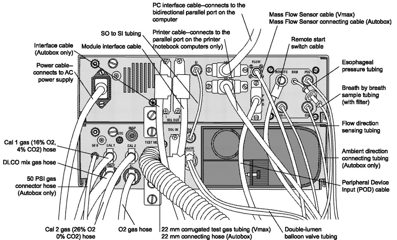
Figure 2-6 – Rear Panel Cables and Tubing—Vmax Analyzer and Pneumatics Modules
