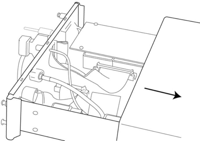
3. Gently remove the cover by sliding it toward the front of the module (Figure 11-2).
