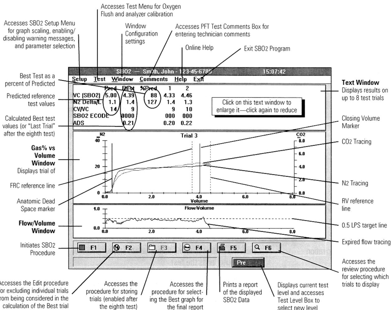
Figure 5-8 – Single Breath Oxygen Test Screen
