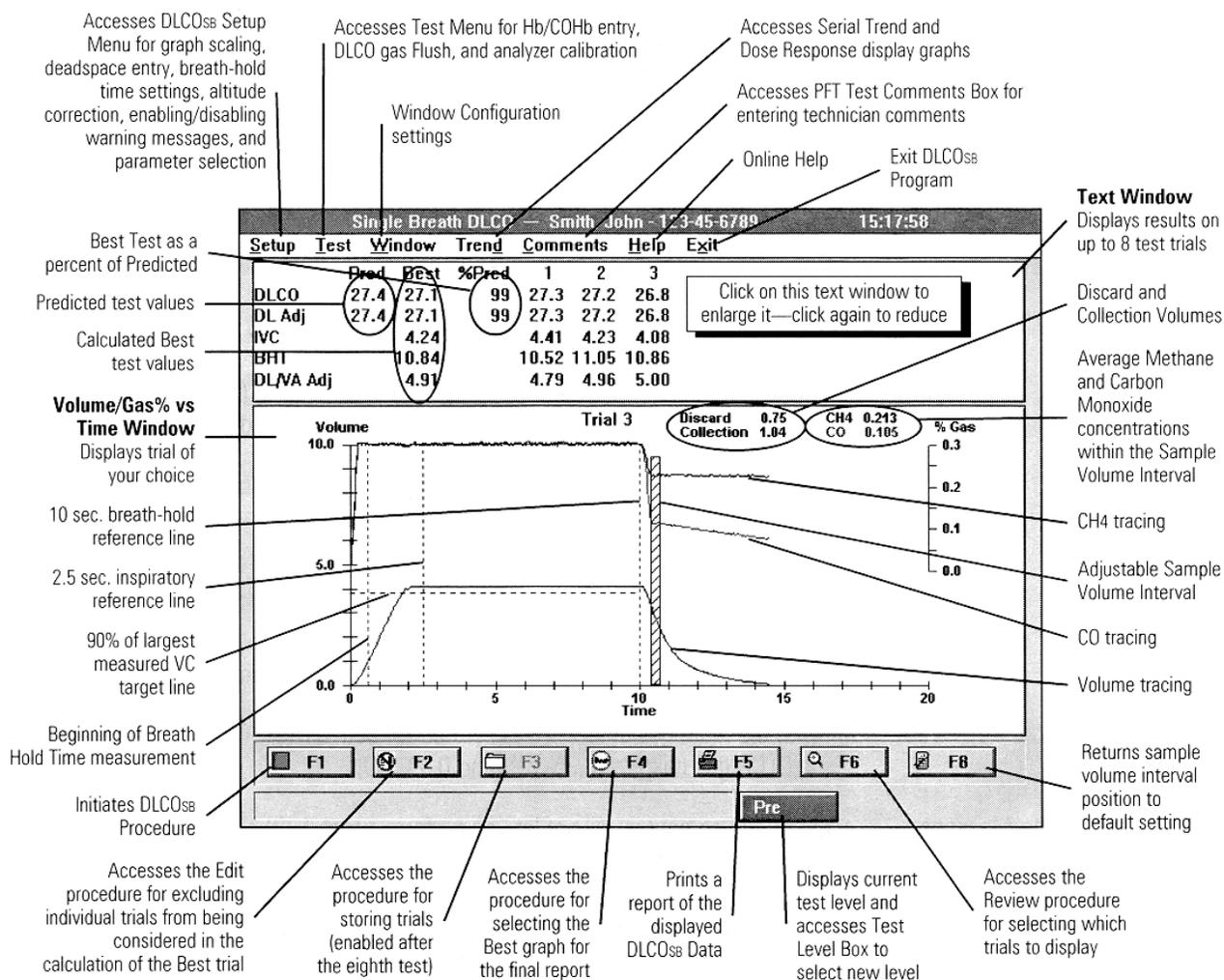
Figure 5-6 – Single Breath DLCO Test Screen
