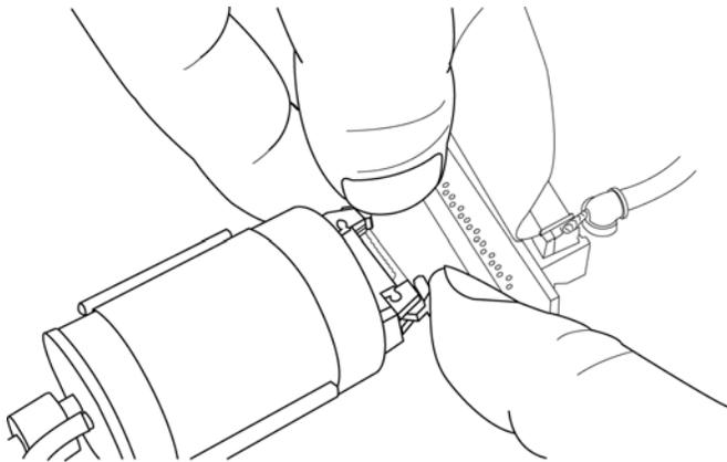
5. Disconnect the ribbon cable by carefully pushing outward on the two locking “ears” of the connector. This connector is on the end of the O<sub>2</sub> sensor (Figure 11-4).
