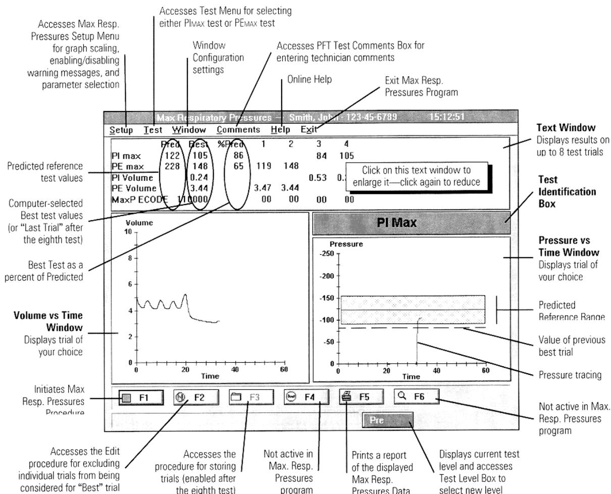
Figure 7-1 – Maximal Respiratory Pressures Test Screen
