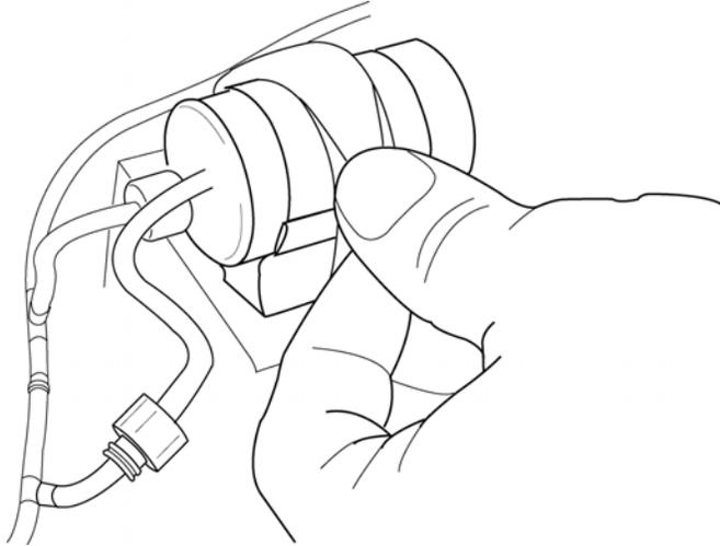
4. Unfasten the strap that secures the O<sub>2</sub> sensor, which is at the front of the module (Figure 11-3).
