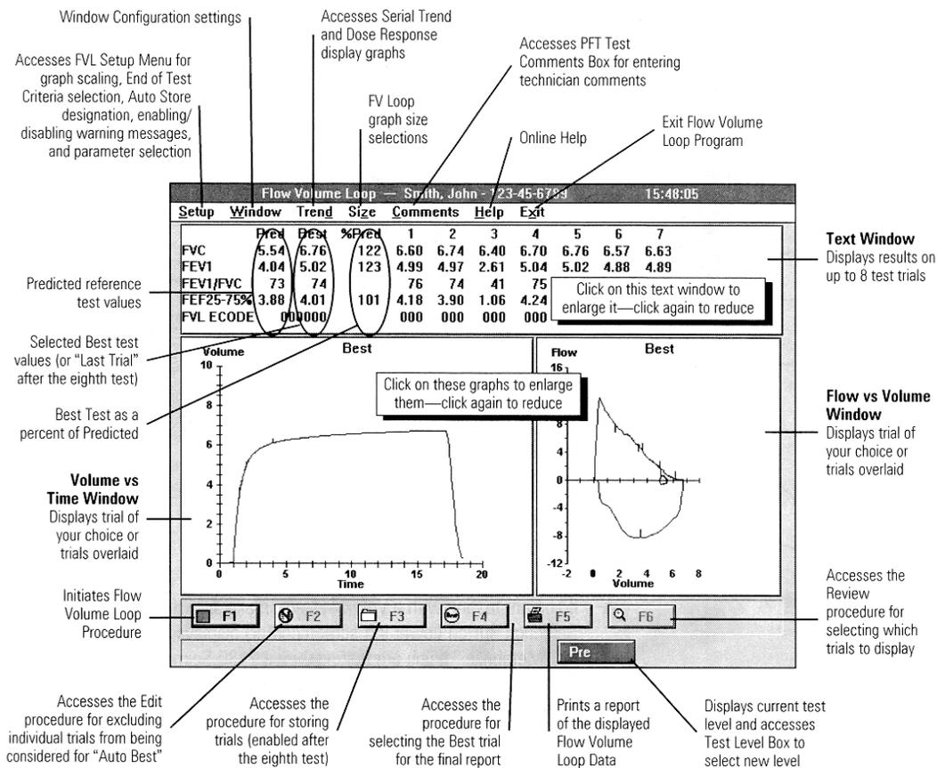
**Figure 5-2 – Flow Volume Loop Test Screen**
