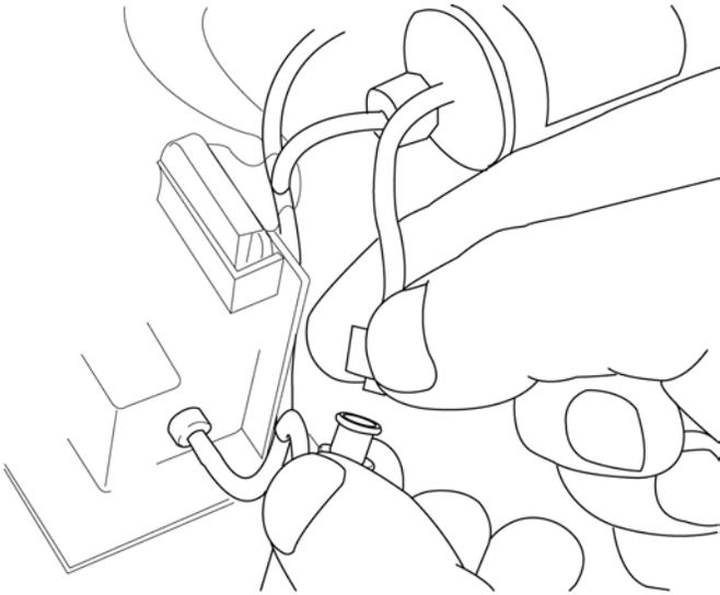
Figure 11-5 – Disconnecting the In-line Luer Fitting
