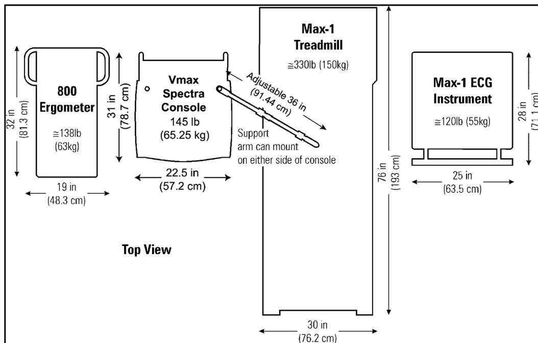
Figure 2-3 – Vmax 229 Pulmonary Function/Cardiopulmonary Exercise Testing Instrument (with Console, Treadmill, Ergometer, and ECG Instrument)
