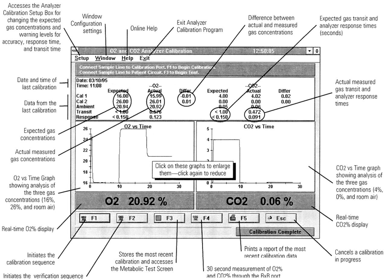
**Figure 8-2 – Analyzer Calibration Screen**
