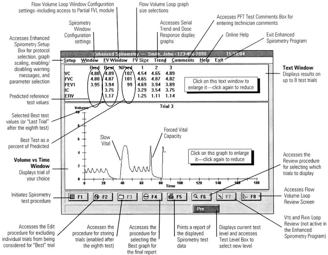
Figure 5-3 – Enhanced Spirometry Test Screen
