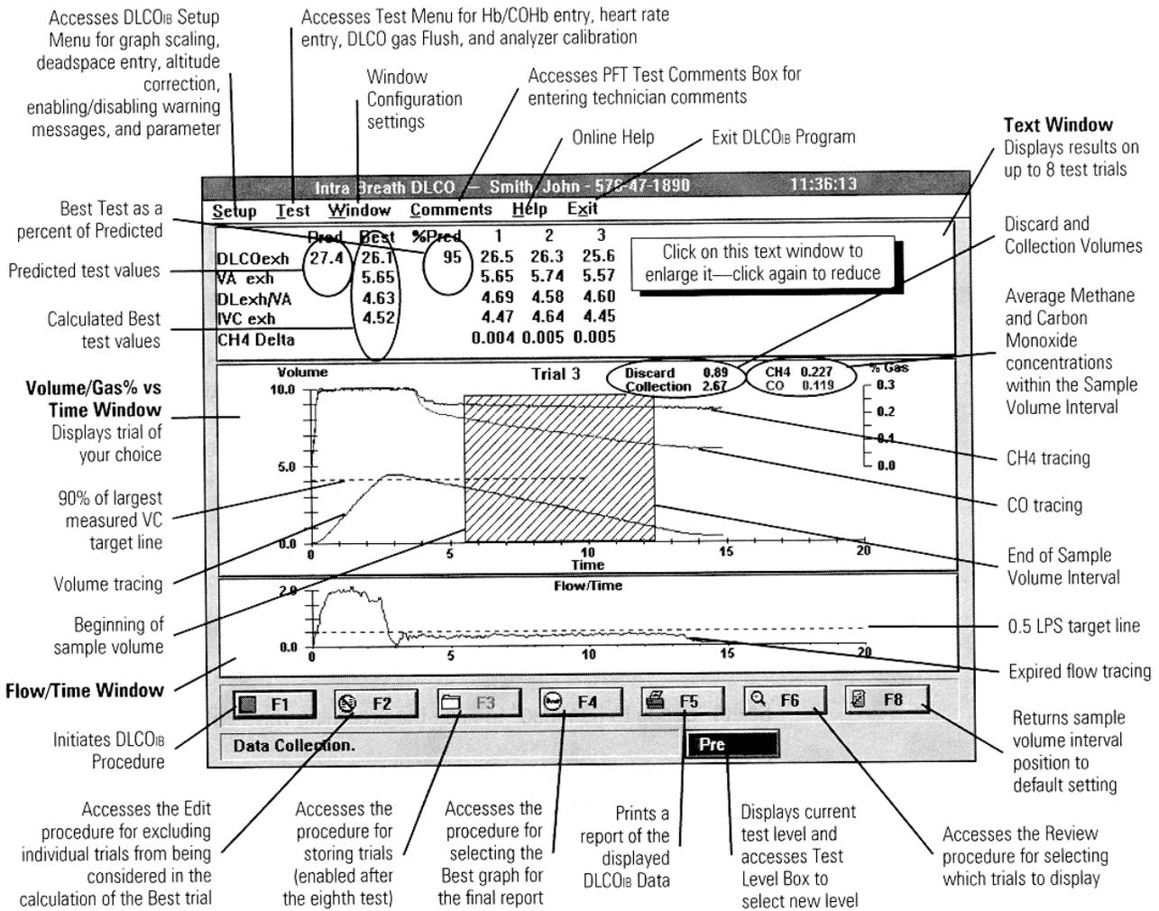
Figure 5-7 – Intra Breath DLCO Test Screen
