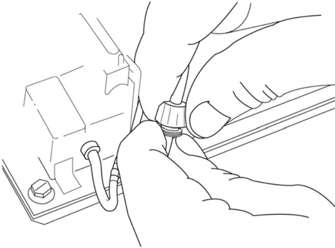
**Figure 11-9 – Reconnecting the In-line Luer Fitting**
