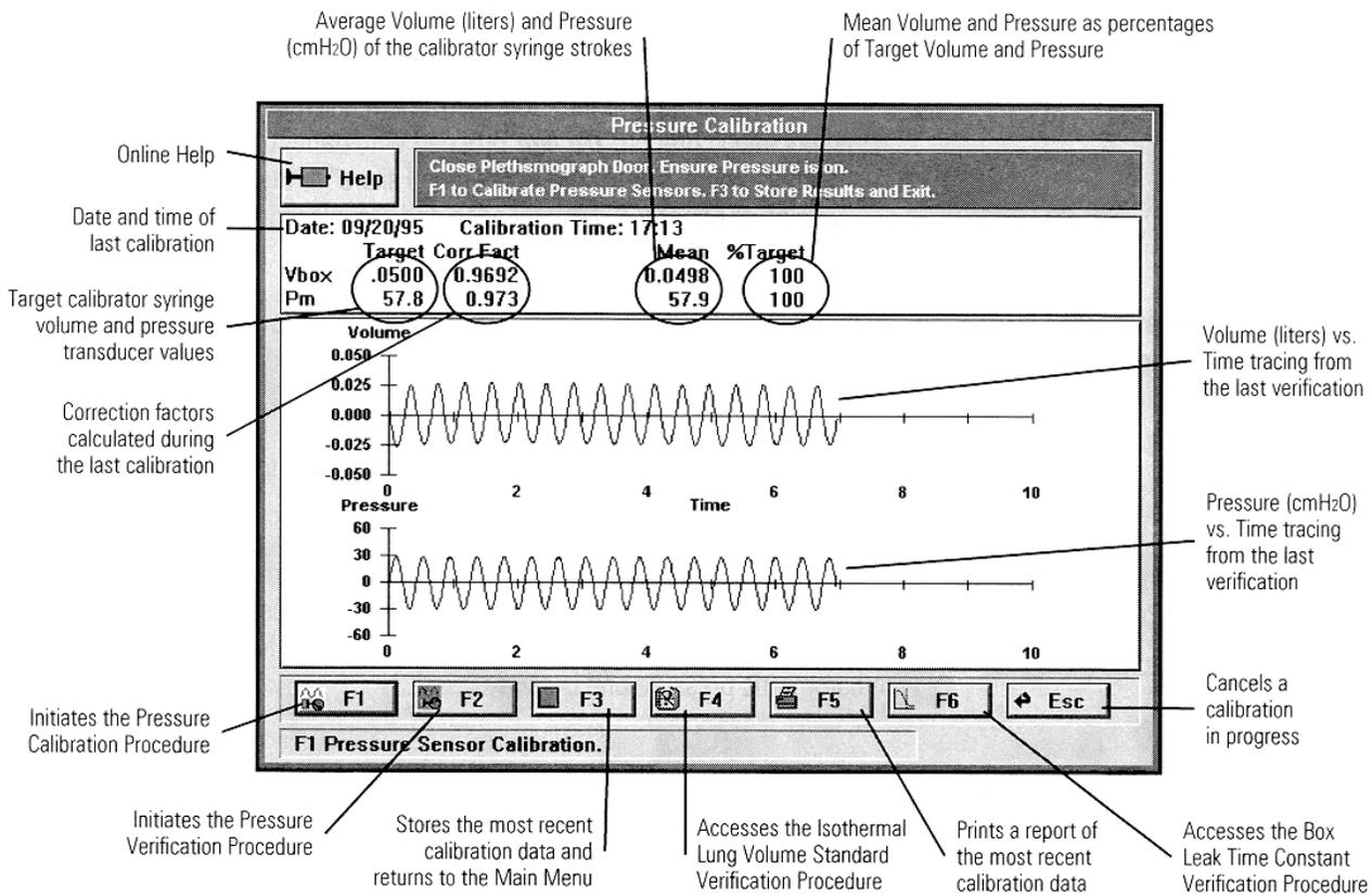
Figure 4-1 – Pressure Calibration Screen
