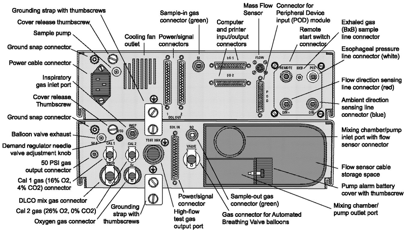
Figure 2-5 – Rear Panel Connectors—Vmax Analyzer and Pneumatics Modules
