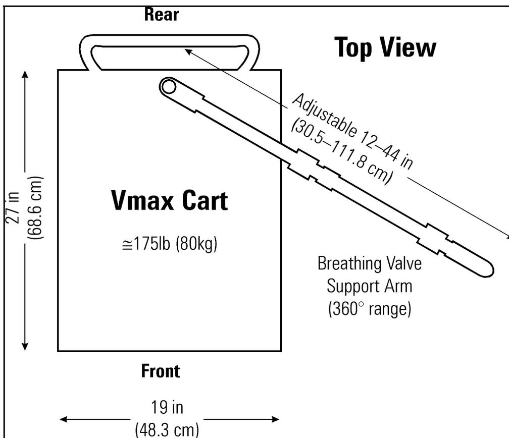
Figure 2-1 – Vmax 22 Pulmonary Function Laboratory (with Cart)
