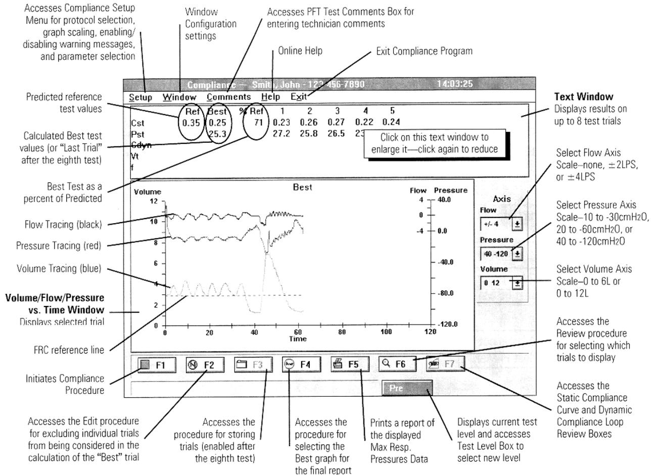
Figure 7-2 – Compliance Test Screen
