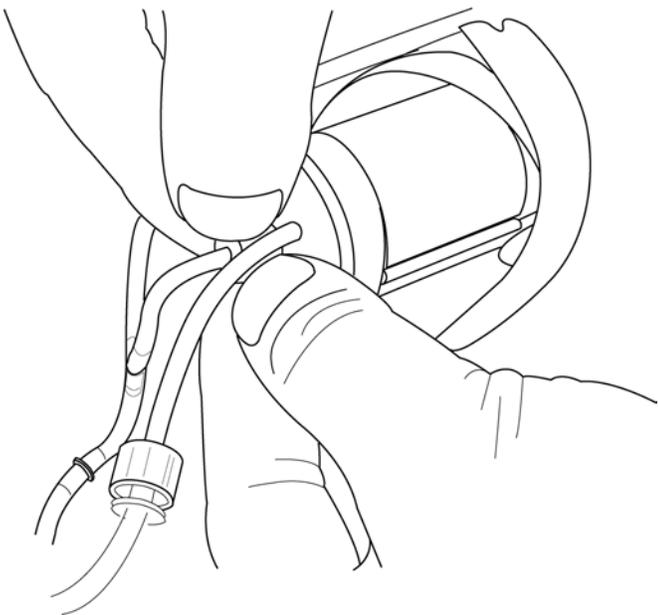
Figure 11-6 – Disconnecting the Luer Fitting
