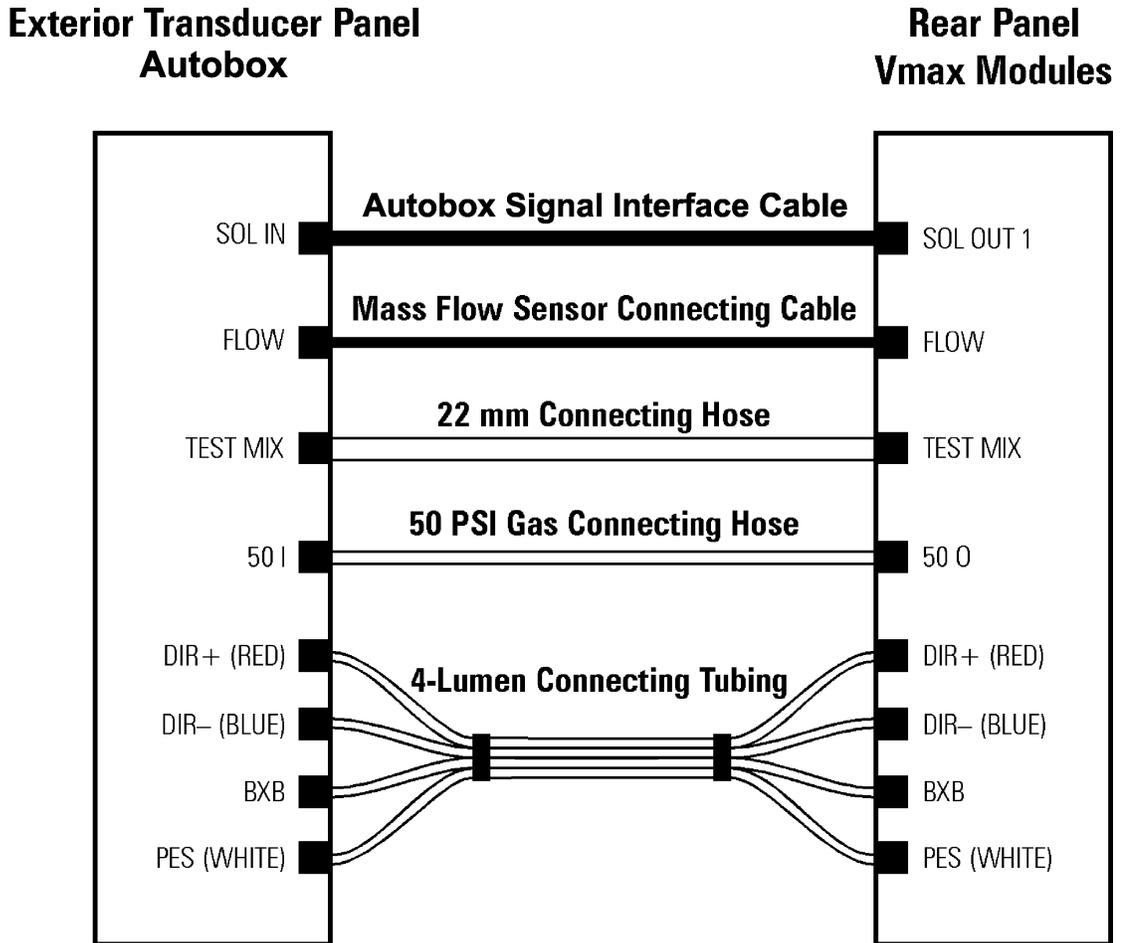
Figure 2-8 – Autobox to Vmax Connections
