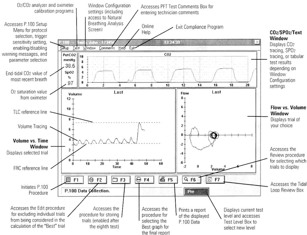
Figure 7-5 – P.100 Test Screen
