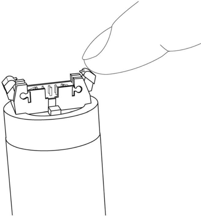
**Figure 11-7 – Connector Locking Ears**
