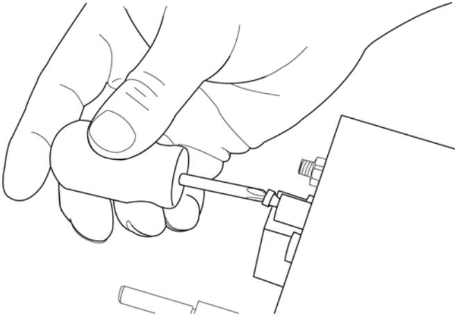
2. Loosen the cover retaining screw that is on the back of the Vmax analyzer (top) module (Figure 11-1).
