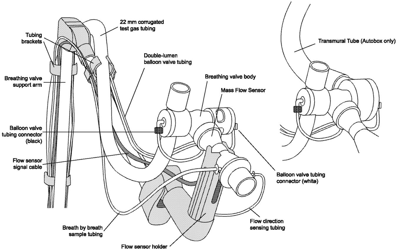
Figure 2-7 – Vmax Breathing Valve and Autobox Breathing Valve with Mass Flow Sensor Connections
